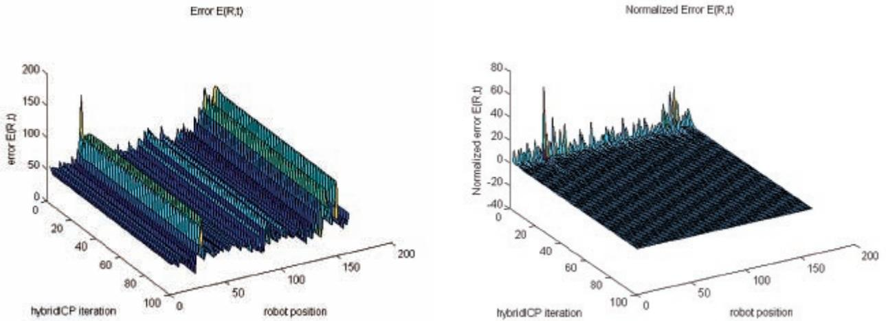
Fig. 3. The error  $E(R, t)$  (see eq. 3) for each robot position in function of hybridICP algorithm iterations
