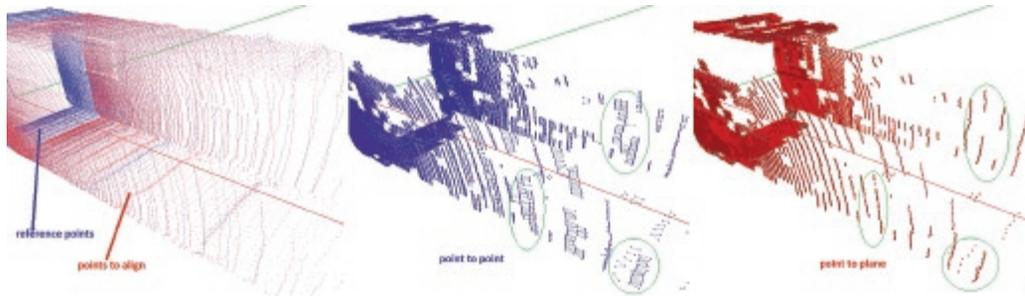
Fig. 1. Comparison between point to point and point to plane methods. In the central image correspond points are connected via line segments. When we are sampling from two different perspectives, we will not in general sample the exact same point. Point to plane method eliminates this problem (green circles)
