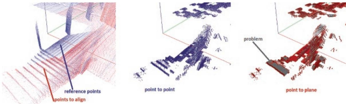
Fig. 5. Problem of point to plane ICP in data containing stairs
