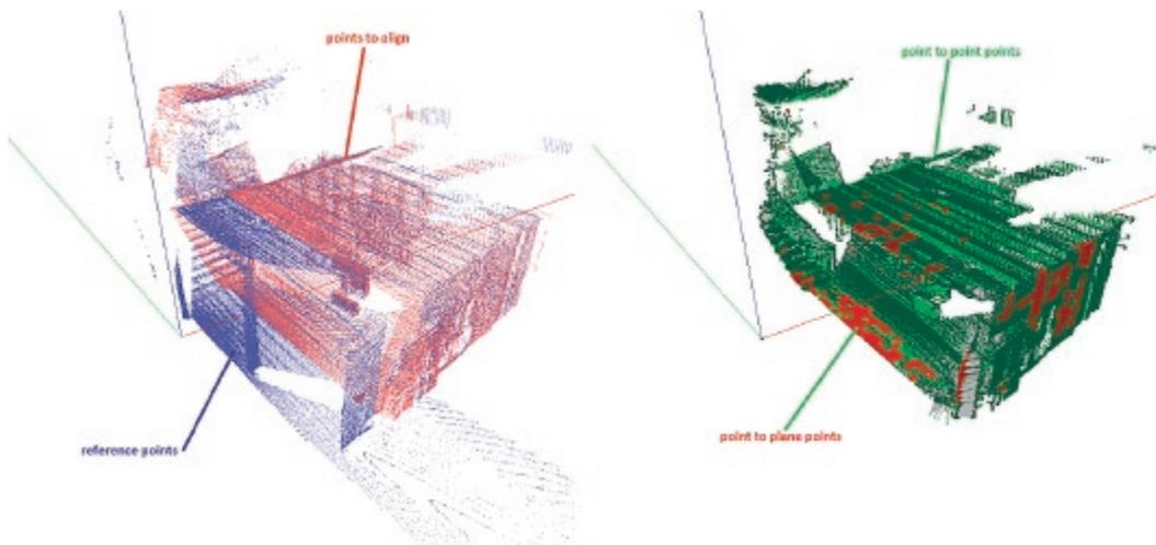
Fig. 7. An example of data set containing 7% of points that were able to be projected during hybrid ICP computation
