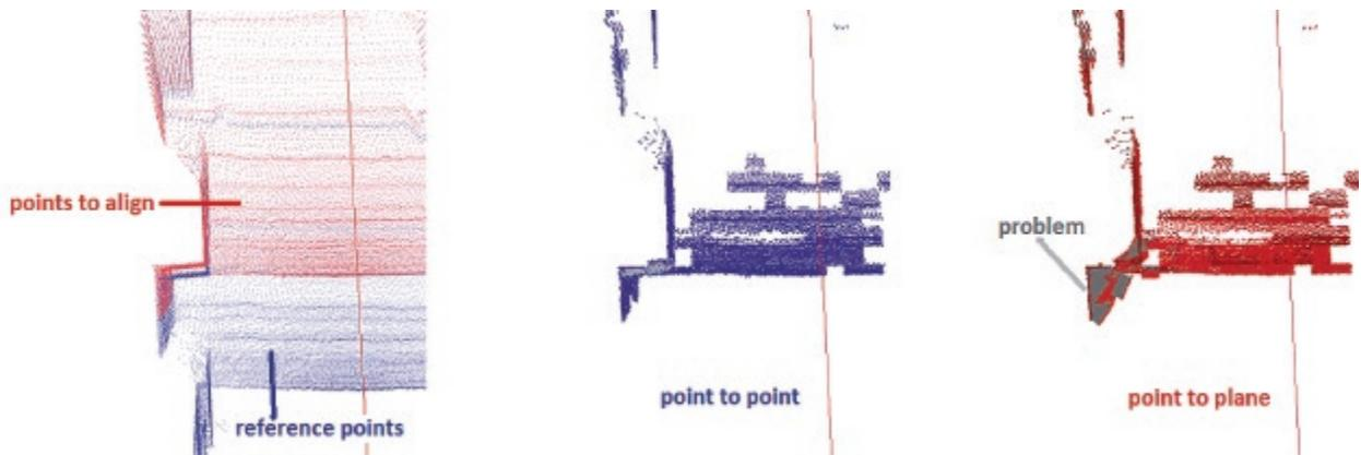
Fig. 6. Problem of point to plane ICP in data containing corner
