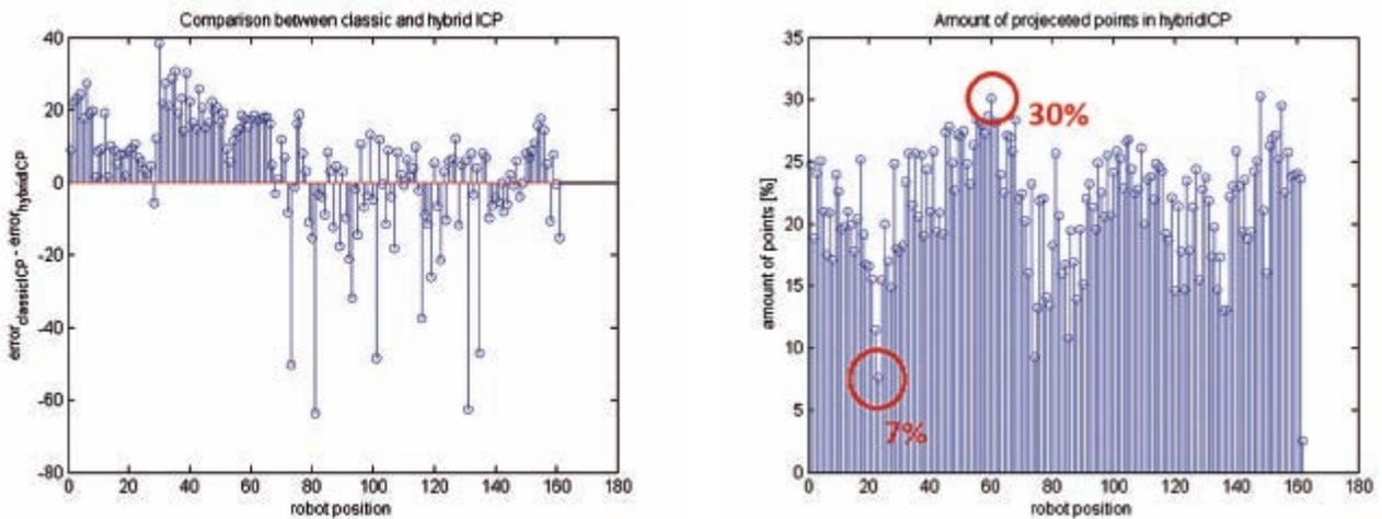
Fig. 4. Left-comparison of classic ICP and hybridICP accuracy. Positive value corresponds to higher accuracy of hybridICP over classic ICP. Right-an amount of points projected onto locally approximated planes in percentage
