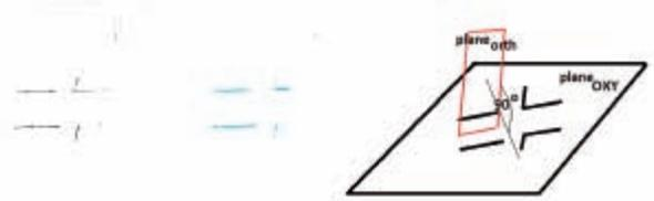
Fig. 5. Walls prerequisites detection. Left: Input image, centre: result as lines (prerequisites of walls), right: example orthogonal plane<sub>orth</sub> to plane<sub>OXY</sub>.
