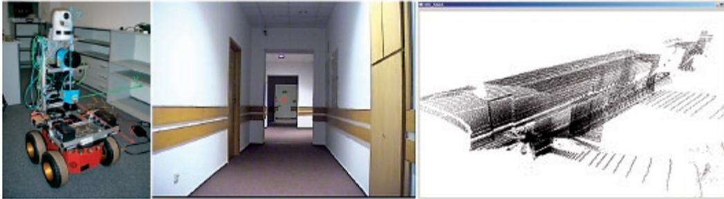
Fig. 1. Robot PIONEER 3AT equipped with SARA (Sensor Data Acquisition System for Mobile Robotic Applications). From left: robot, image from onboard camera, 3D cloud of points
