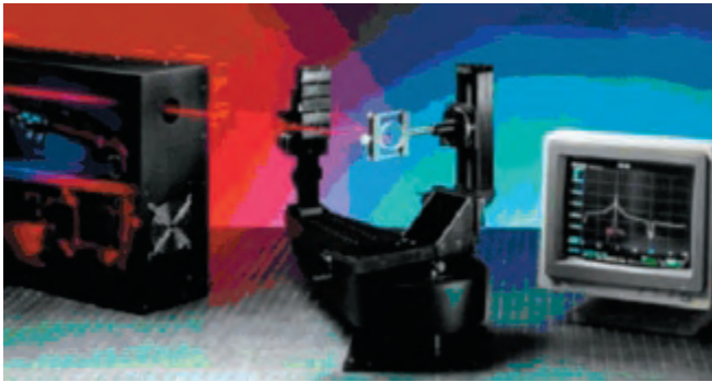
Rys. 4. Skaterometr CASI firmy Schmitt Measurement Systems Inc Fig. 4. The Schmitt measurement Systems Inc. Casi Scatterometer
