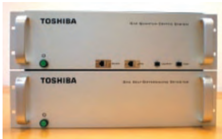
Rys. 3. Serwer klucza kwantowego w łączu Toshiba Fig. 3. Quantum Key Server consists of two compact boxes designed to fit into a communications rack ( http://www.toshiba-europe.com/research/crl/qig/quantumkeyserver.html )
